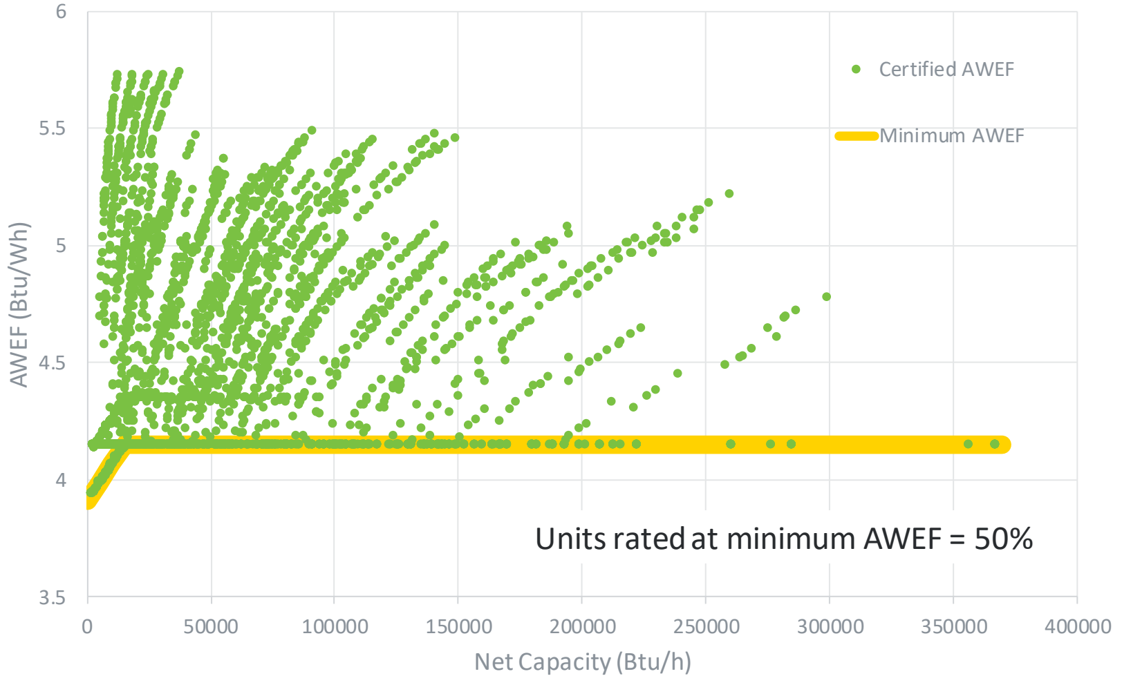
Market Snapshot - Low Temperature Unit Coolers As of February 2, 2021
