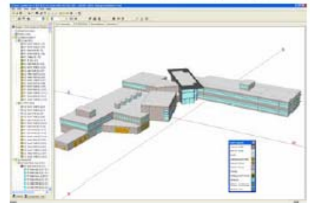
Whole-building energy model in eQuest
